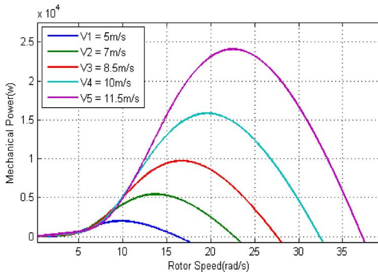
Figure 2. Power-speed curve of wind turbine
