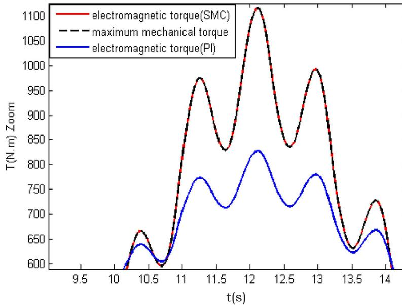
Figure 7. PMSG electromagnetic torque in zoom mode
