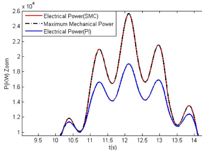
Figure 5. PMSG electric power in zoom mode
