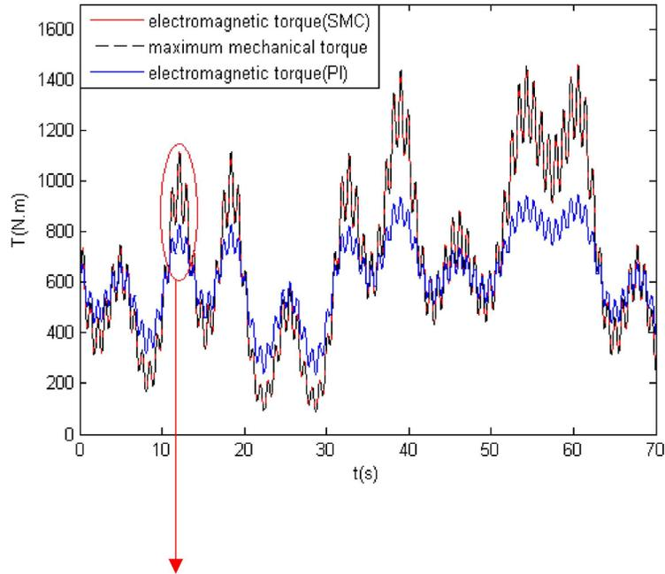
Figure 6. PMSG electromagnetic torque
