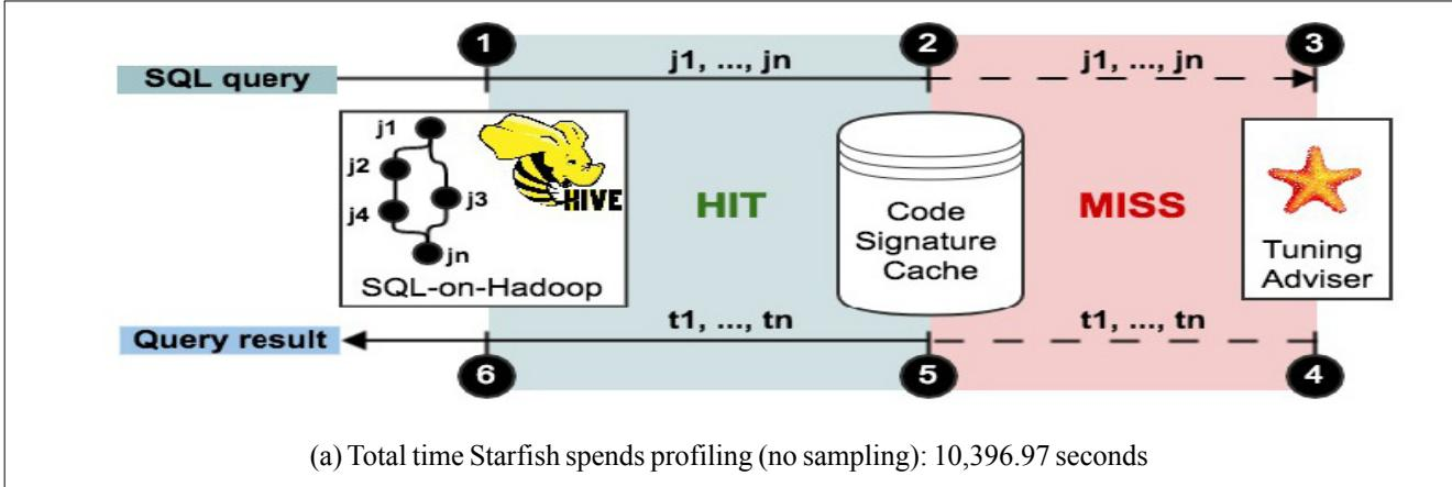
Figure 1. The DejaVu code signature cache. Jobs  $j_i$  are mapped to tuning setups  $t_i$ , using the code signature as cache key
