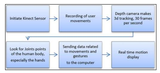
Figure 2. Structure of the interaction of the Kinect device
