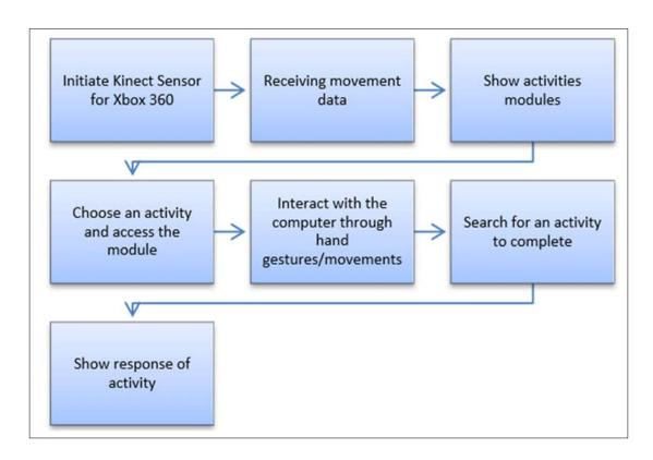
Figure 3. Structure of the System with the Kinect device
