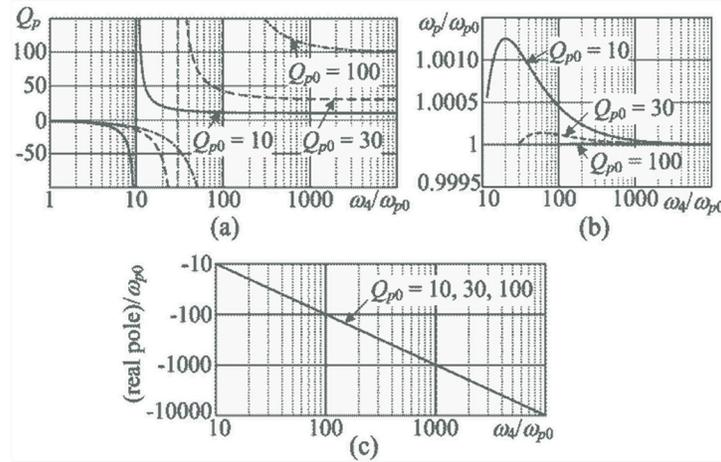
Figure 2. Influence of the ratio  $\omega_4/\omega_{p0}$  for the circuits in Figure 1(c), (d) and (e): (a) change of the pole Q-factor; (b) change of the pole frequency; (c) extra real pole
