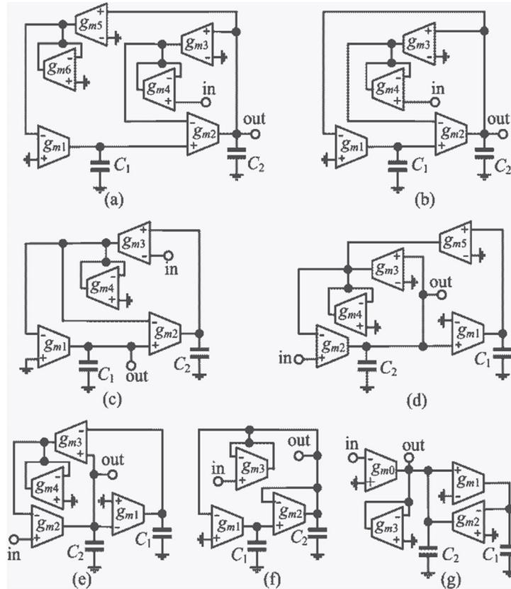
Figure 1. Two-integrator loop biquads [1]: (a), (b), (c) distributed feedback configurations; (d), (e) summed-feedback configurations; (f) Tow-Thomas Gm-C circuit; (g) gyrator band-pass biquad
