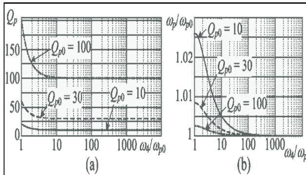
Figure 3. Influence of parasitic frequency  $\omega_4 = g_{m4}/C_{p4}$  in Figure 1(b): (a) variation of pole Q-factor; (b) variation of pole frequency  $\omega_4$
