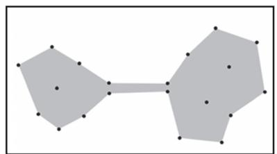
Figure 3. An  $\alpha$ -shape that generates a narrow bridge between two point sets
