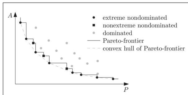
Figure 2. Different types of solutions and Pareto-frontier of a bicriteria optimization problem
