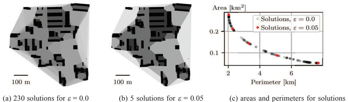
Figure 7. Solutions obtained with Algorithm 1 for the same instance without (a) and with approximation (b) and their values for the two objectives (c). Darker polygons correspond to solutions for higher  $\alpha$  values, which consist of multiple groups
