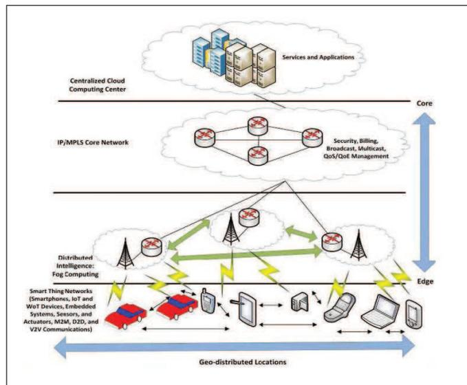
Figure 1. Fog Computing Architecture
