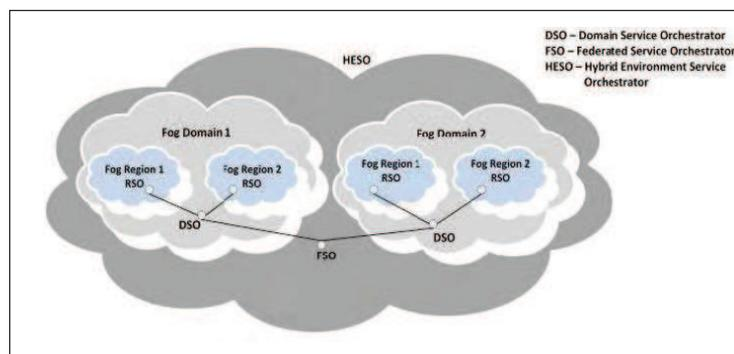
Figure 2. Hybrid Environment Service Orchestrator Model for Fog Computing
