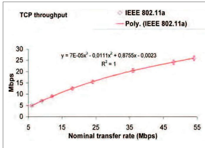
Figure 4. TCP throughput versus technology and nominal transfer rate; Open, PTP
