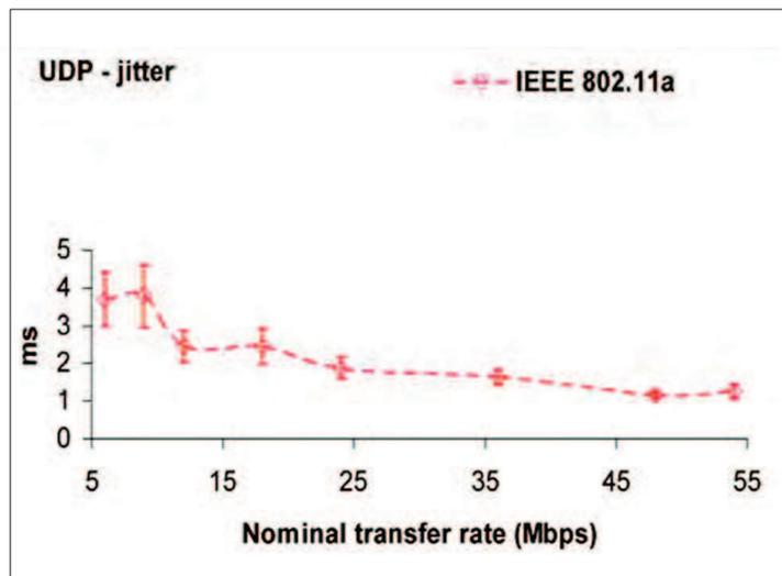
Figure 5. UDP - jitter results versus technology and nominal transfer rate; WPA, PTP
