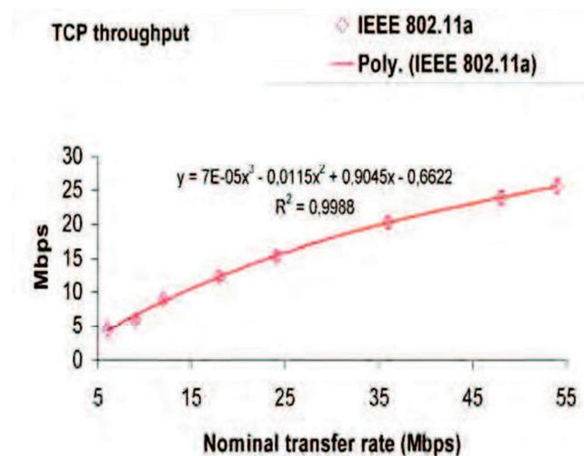
Figure 3. TCP throughput versus technology and nominal transfer rate; WPA, PTP
