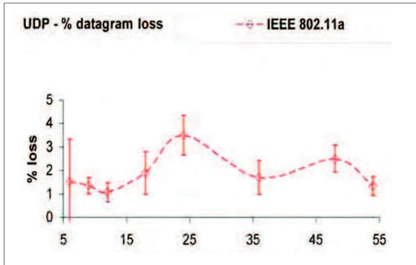
Figure 7. UDP – percentage datagram loss versus technology and nominal transfer rate; WPA, PTP
