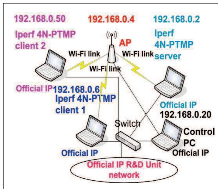
Figure 1. Wi-Fi laboratory setup scheme
