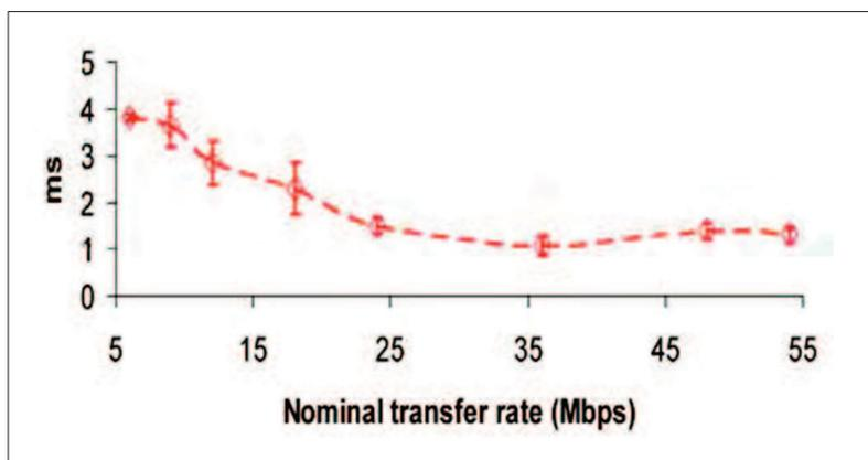
Figure 6. UDP - jitter results versus technology and nominal transfer rate; Open, PTP
