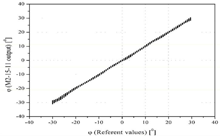
Figure 4. Scattering diagram of MLP2-15-11 model  $\tilde{O}$  output
