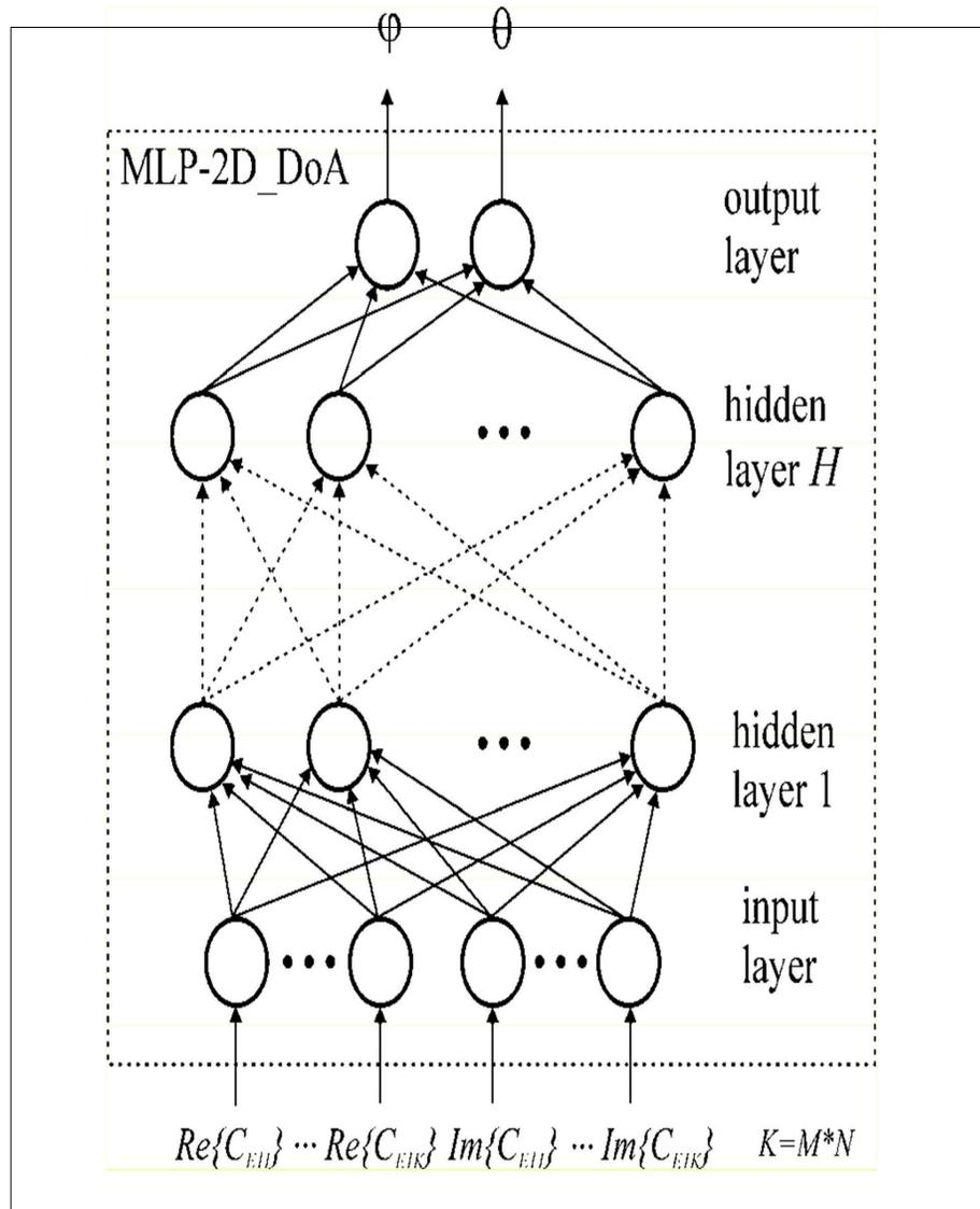
Figure 2. Architecture of MLP neural model for 2D DOA estimation of stochastic EM source signal in  $x$ - $y$  plane plane
