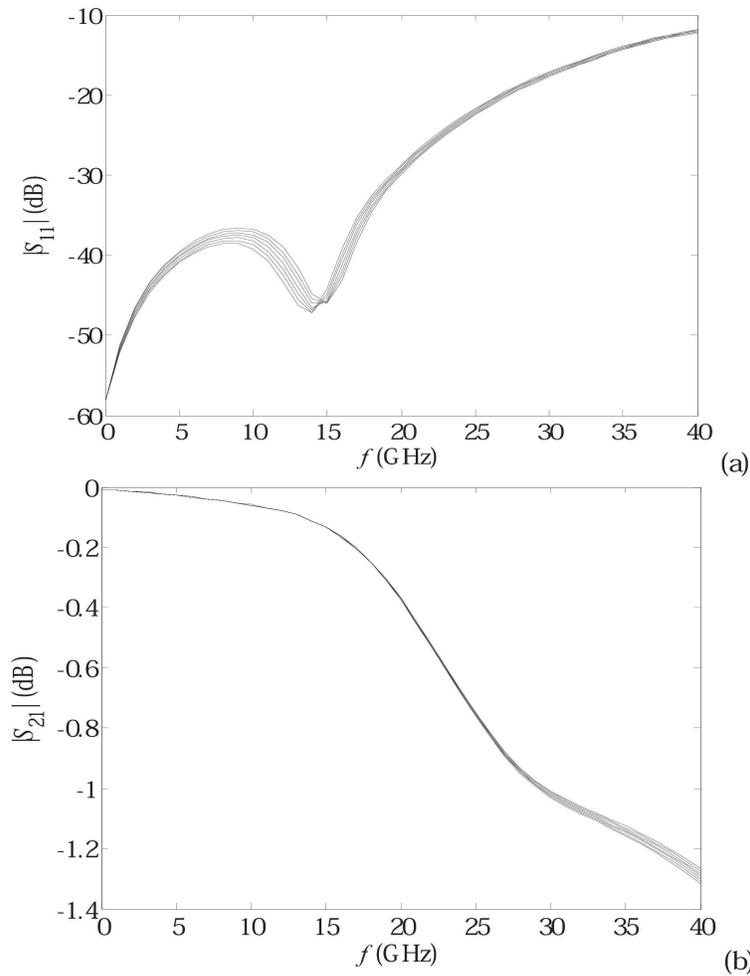
Figure 4. Maximum influence of  $W_b$  deviation: (a) Return loss: device (400, 20, 30, 150), (b) Insertion loss: device (800, 20, 50, 110).
