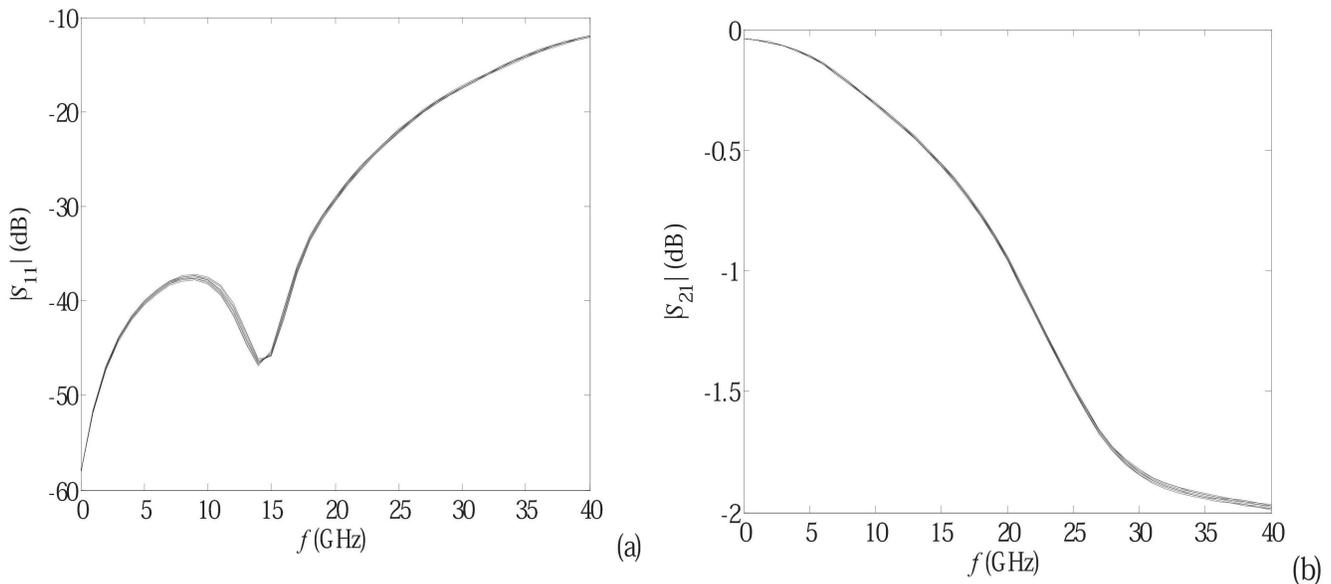
Figure 3. Maximum influence of  $L_b$  deviation: (a) Return loss: device (400, 20, 30, 150), (b) Insertion loss: device (1000, 220, 30, 20)
