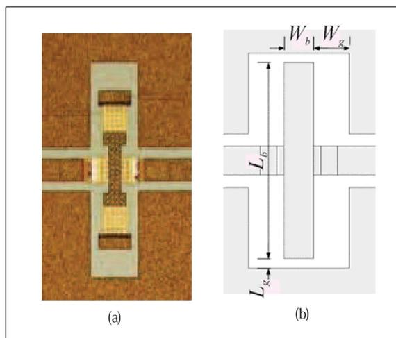
Figure 1. Fabricated ohmic series RF MEMS switch [9] (a) and the simplified configuration (b)
