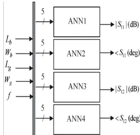
Figure 2. ANN model of ohmic series RF MEMS switch
