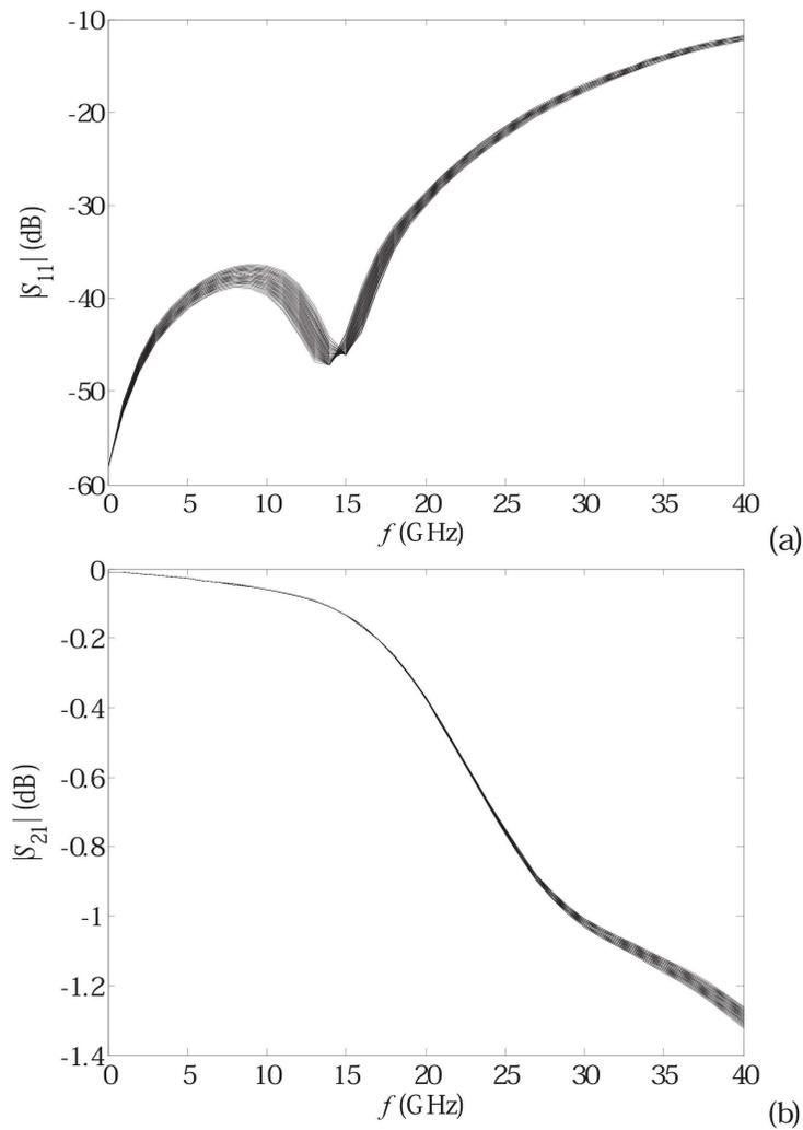
Figure 5. Maximum influence for simultaneously deviation of  $L_b$  and  $W_b$ : (a) Return loss - device (400, 20, 30, 150), (b) Insertion loss - device (800, 20, 50, 110)
