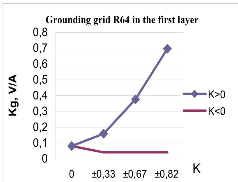
Figure 9.  $K_G$  versus K for R64 100x200
