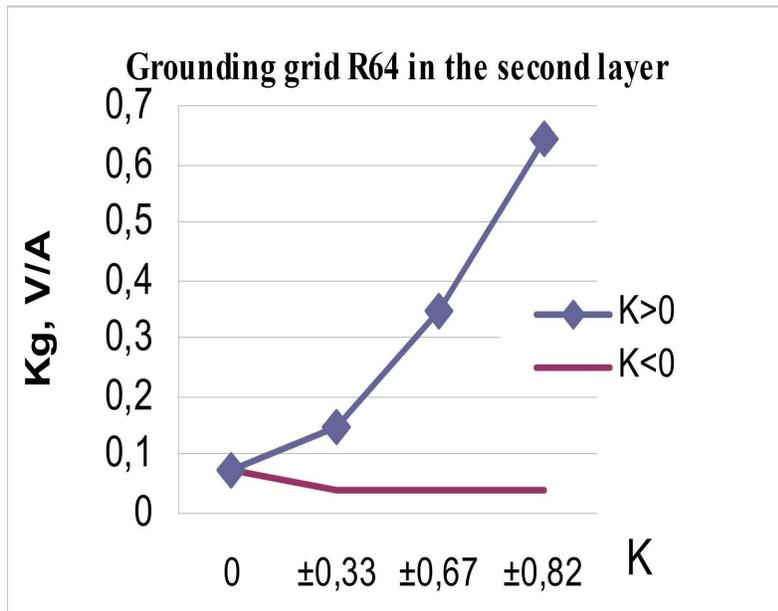
Figure 11.  $K_G$  versus  $K$  for R64 100x200
