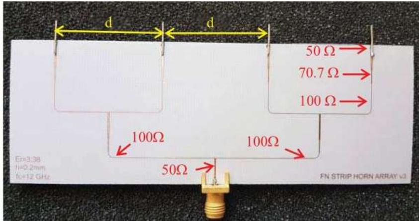
Figure 3. Photograph of the microstrip feed network for the linear array of strip horn antennas (with indicated impedances)
