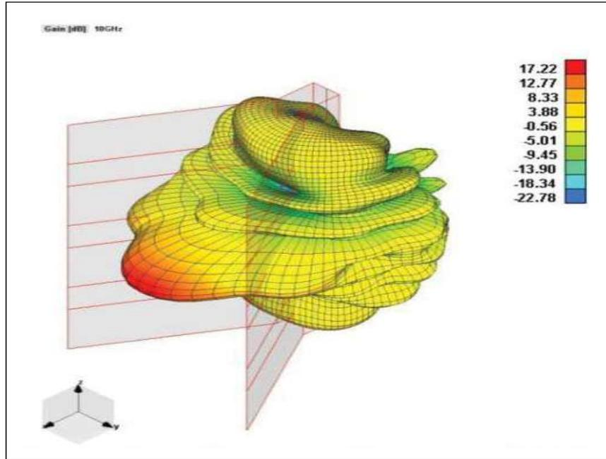
Figure 5. 3D radiation pattern of the proposed linear array of strip horn antennas
