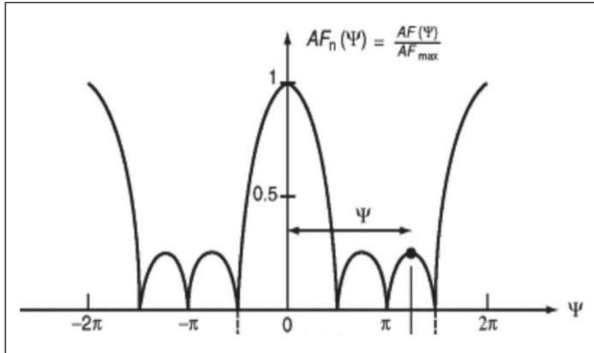
Figure 1. Graphical representation of the normalized array factor of the 4-element array as a function of  $\psi$
