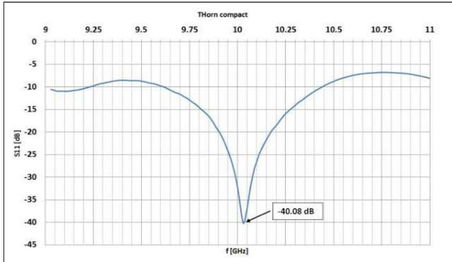
Figure 7. Measured reflection coefficient S11 of the realized strip horn antenna array
