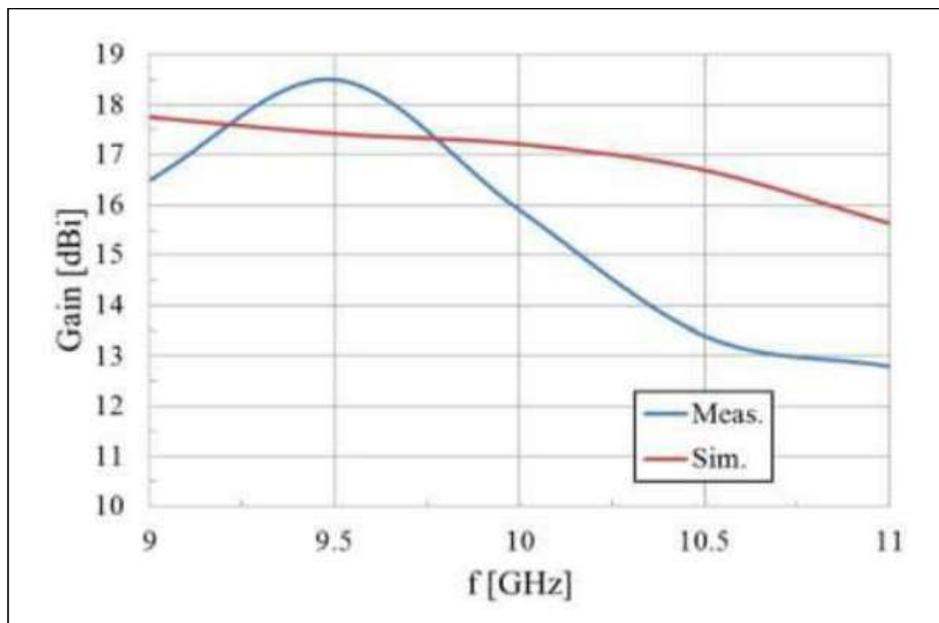
Figure 8. Measured and simulated gains of the realized strip horn compact antenna array
