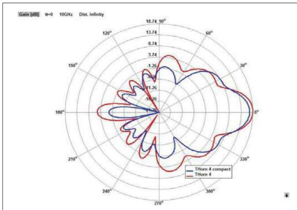
Figure 4. Radiation patterns of the linear array of strip horn antennas in  $xOy$ -plane: individual horns (red line) and with the common reflector (blue line)
