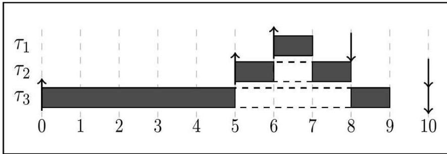
Figure 3. Example schedule showing how the scheduler chooses which task should execute. Task “3” is released at  $t = 0$ . At  $t = 5$ , task “2” is released, pre-empting “3” as although it has the same absolute deadline, it has a lower task index. At  $t = 6$ , task “1” is released, pre-empting task “2”. At  $t = 7$ , “1” completes, the scheduler then chooses to resume task “2” as although it has the same absolute deadline as task “3”, it has the lower task index.
