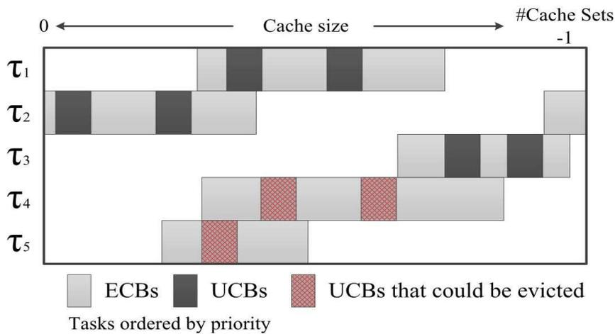
Figure 5. Example layout showing how the position of tasks in cache affects whether their UCBs could be evicted during a pre-emption
