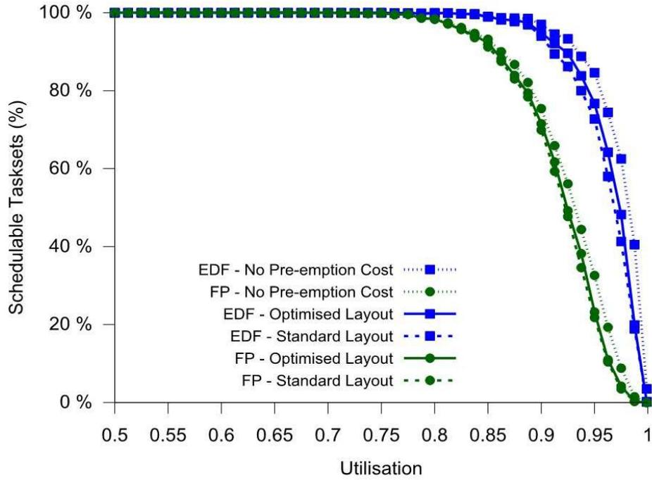
Figure 7. Percentage of schedulable tasksets at each utilisation level for the Mälardalen and SCADE benchmarks for tasksets of cardinality 10
