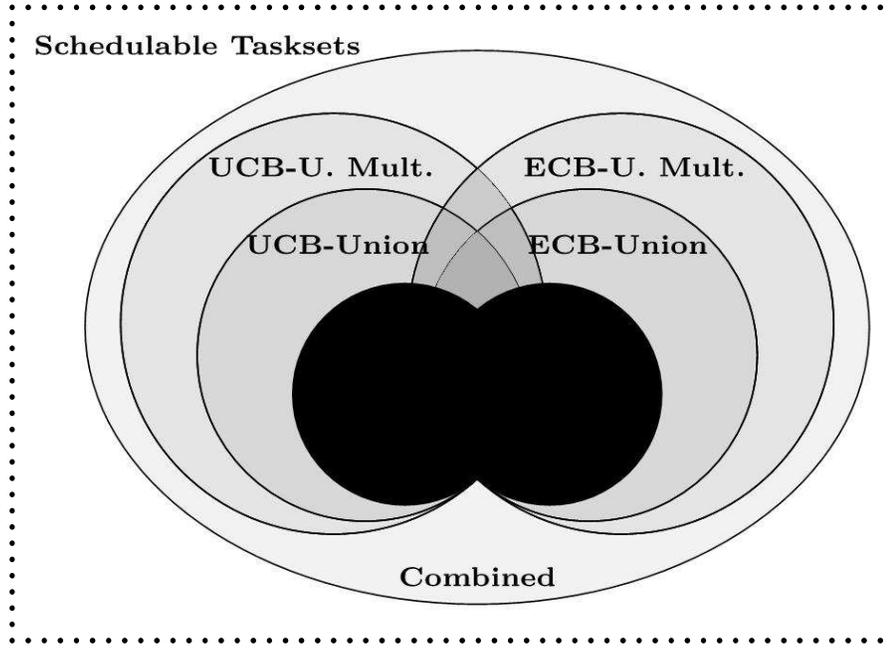
Figure 2. Venn diagram showing the relationship between different approaches for CPRD analysis under FP scheduling.
