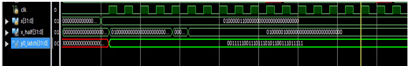
Figure 11. Clock by clock waveform testing of x_{half} and y_0 signals
