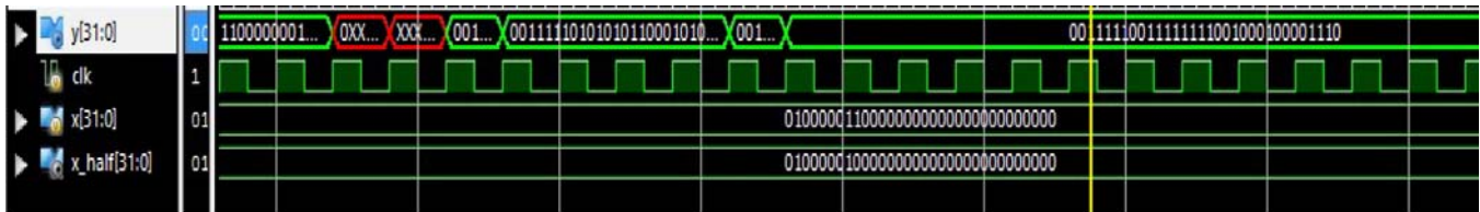
Figure 10. Signal waveform when input at x is 16 (fixed point)
