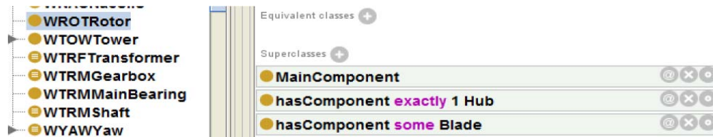
Figure 3. WROTRotor class is a subclass of a class which is a MainComponent class and has Blade and Hub as components
