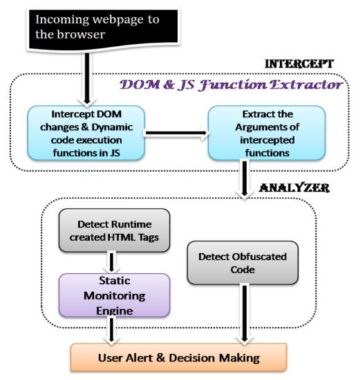
Figure 6. Architecture of Runtime Monitoring Engine
