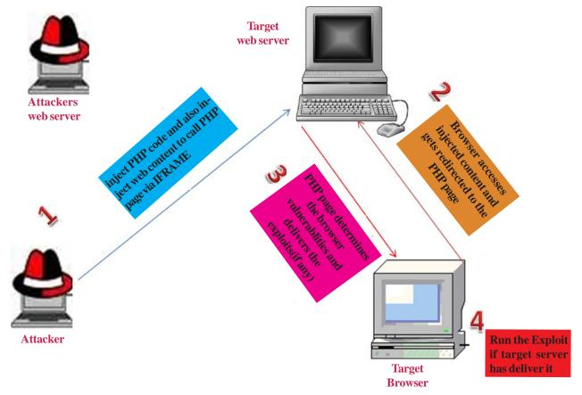
Figure 1. Drive by Download attack scenario - Exploit code resides on Target server
