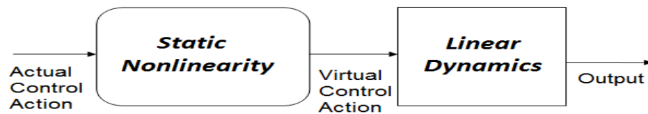
Figure 6. Structure of Hammerstein model
