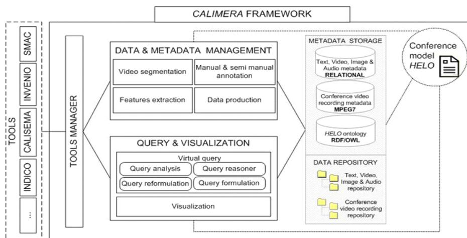
Figure 2. CALIMERA architecture detailed view
