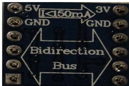
Figure 2. Bi-directional Logic Level Converter
