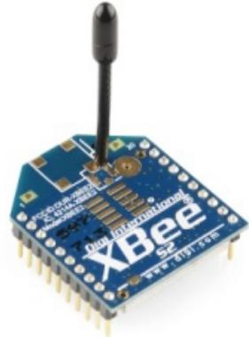
Figure 5. XBee series 2 module
