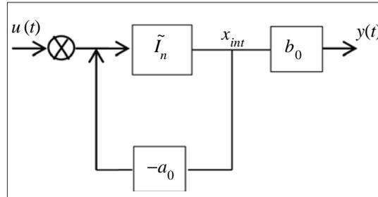
Figure 2. Block representation scheme of non-integer system ( $0 < n < 1$ )
