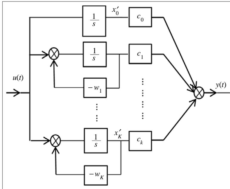
Figure 2. The modal representation (Infinite State representation) of fractional integrator
