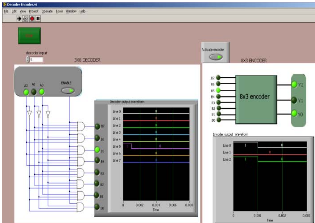
Figure 7. Decoder Encoder when the input is 101
