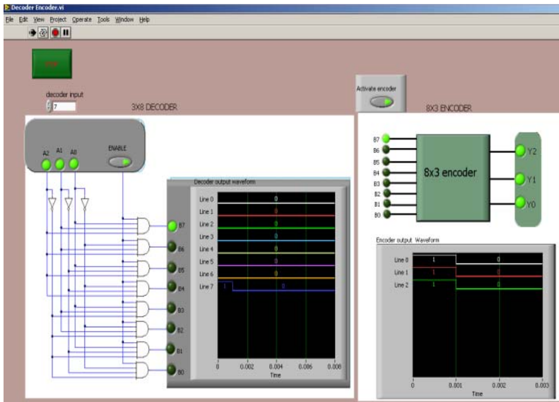
Figure 8. Decoder Encoder when the input is 111
