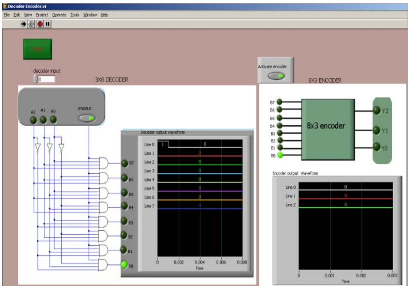
Figure 4. Decoder Encoder when the input is 000
