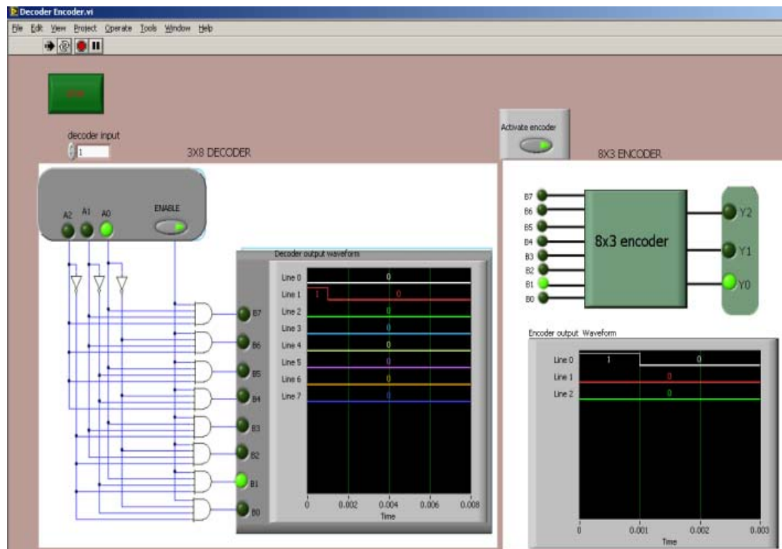
Figure 6. Decoder Encoder when the input is 011
