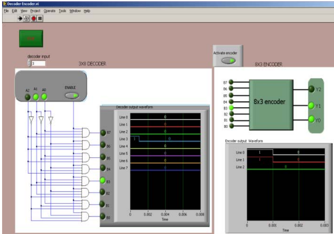
Figure 5. Decoder Encoder when the input is 001
