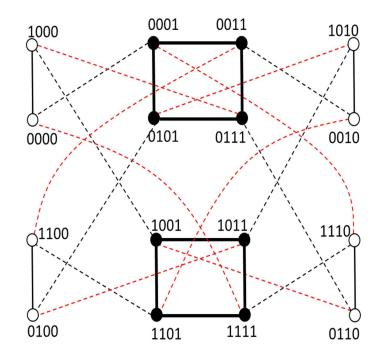
Figure 2. An exchanged folded hypercube EFH(1,2)
