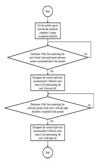
Figure 2. Flowchart of utilizing the notebook computer's image recognition function to calibrate the necklace's internal parameters
