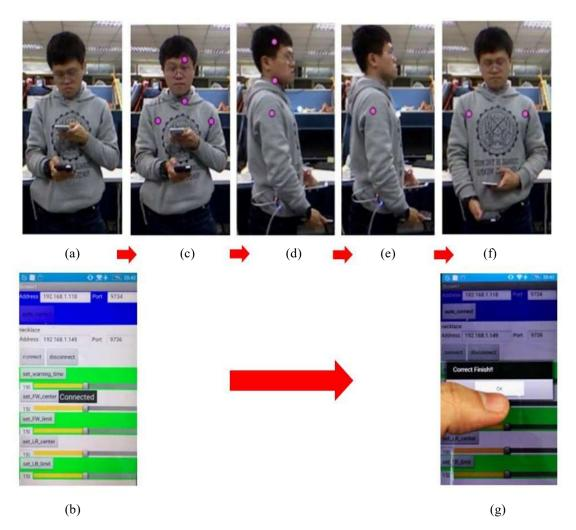
Figure 4. Using the notebook computer's image recognition function to calibrate the necklace's internal parameters
