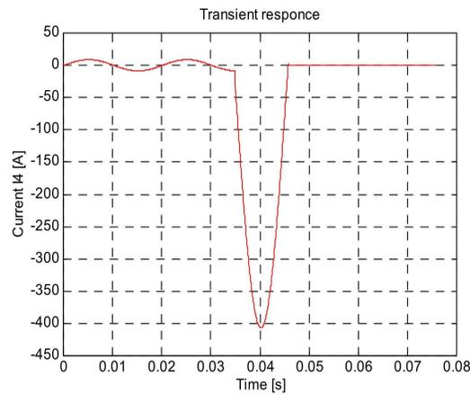
d) Simulation of the current through switch  $\kappa_4 - i_4(t)$  at  $\varphi = 270^\circ$
