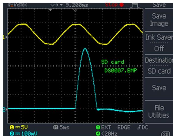
c) Oscillogram of the current through switch  $\kappa_3 - i_3(t)$  at  $\varphi = 270^\circ$
