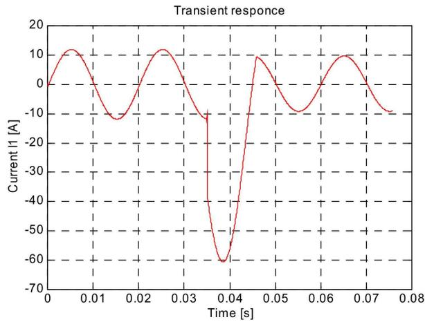
a) Simulation of the input current  $i_1(t)$  at  $\varphi = 270^\circ$
