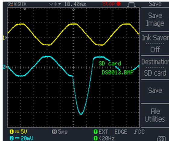
a) Oscillogram of the input current  $i_1(t)$  at  $\varphi = 270^\circ$
