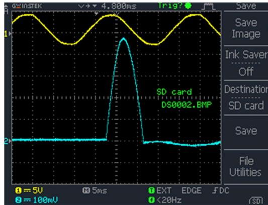
b) Oscilloscope of the current through switch  $\kappa_3 - i_3(t)$  at  $\varphi = 225^\circ$
