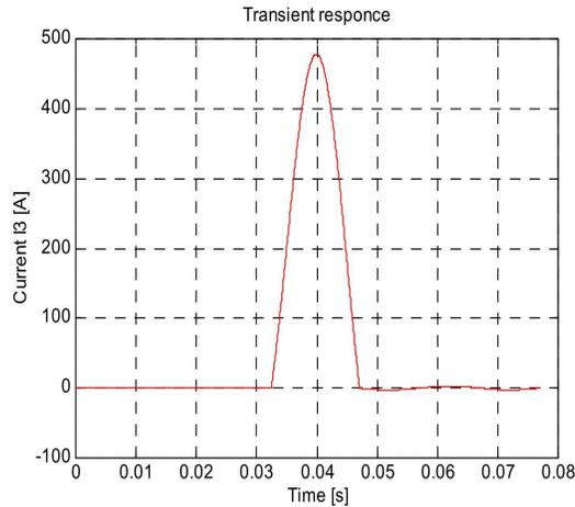
b) Simulation of the current through switch  $\kappa_3 - i_1(t)$  at  $\varphi = 225^\circ$
