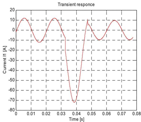
a) Simulation of the input current  $i_1(t)$  at  $\varphi = 225^\circ$
