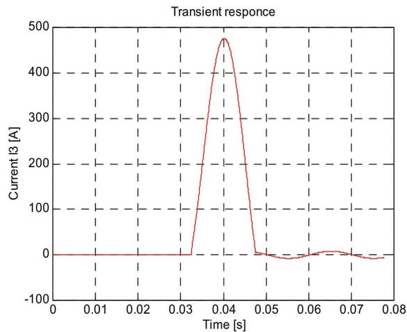
b) Simulation of the current through switch  $\kappa_3 i_3(t)$  at  $\varphi = 225^\circ$
