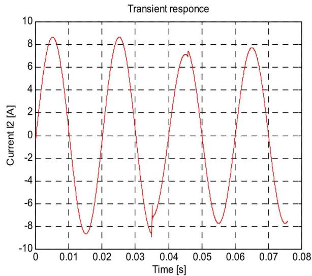
b) Simulation of the output current  $i_2(t)$  at  $\varphi = 270^\circ$
