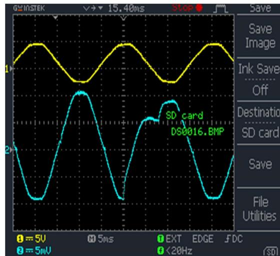
b) Oscillogram of the output current  $i_2(t)$  at  $\varphi = 270^\circ$
