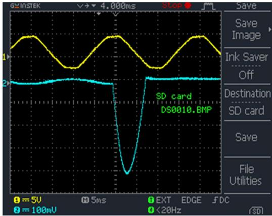
d) Oscillogram of the current through switch  $\kappa_4 - i_4(t)$  at  $\varphi = 270^\circ$
