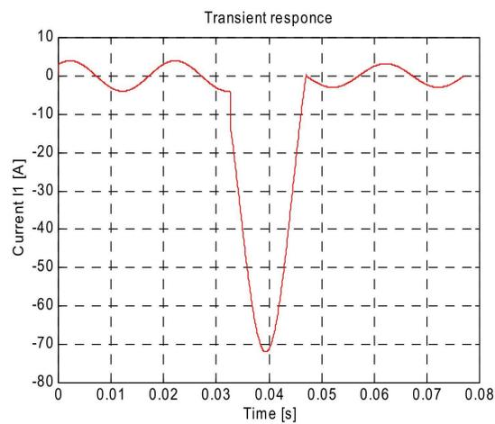
a) Simulation of the input current  $i_1(t)$  at  $\varphi=225^0$
