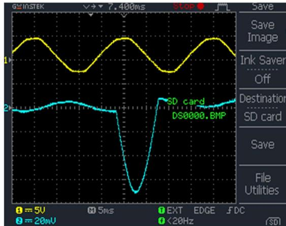
a) Oscillogram of the input current  $i_1(t)$  at  $\varphi=225^0$
