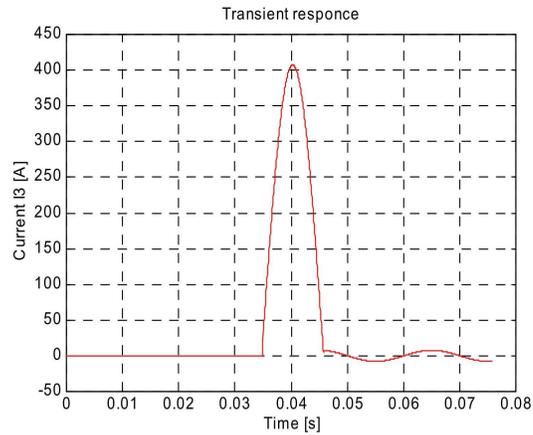
c) Simulation of the current through switch  $\kappa_3 - i_3(t)$  at  $\varphi = 270^\circ$
