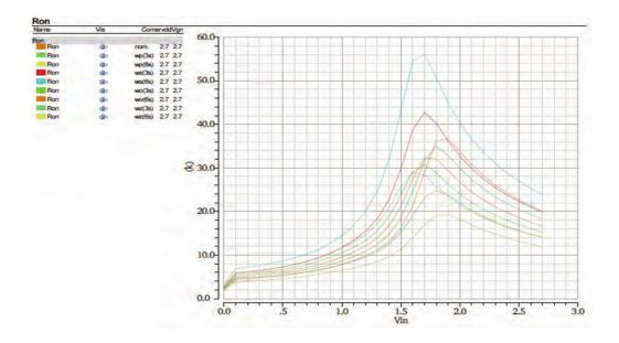
Figure 3. Corner analyses of the transmission gate
