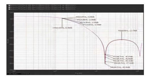
Figure 7. Frequency response of the filter – PAC corner analyses
