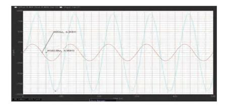
Figure 9. Transient response of the filter for group delay verification typical conditions (27°C, VDD = 3V)
