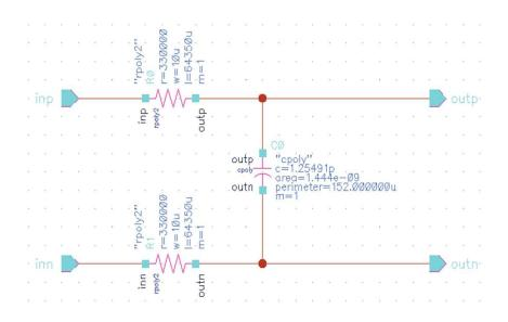
Figure 5. Anti-aliasing filter schematic in Cadence® Virtuoso®
