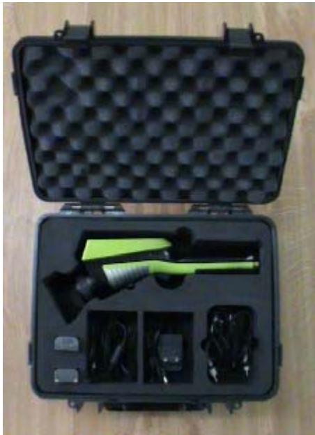
Figure 2. ULIRVision TI160 thermal imaging camera
