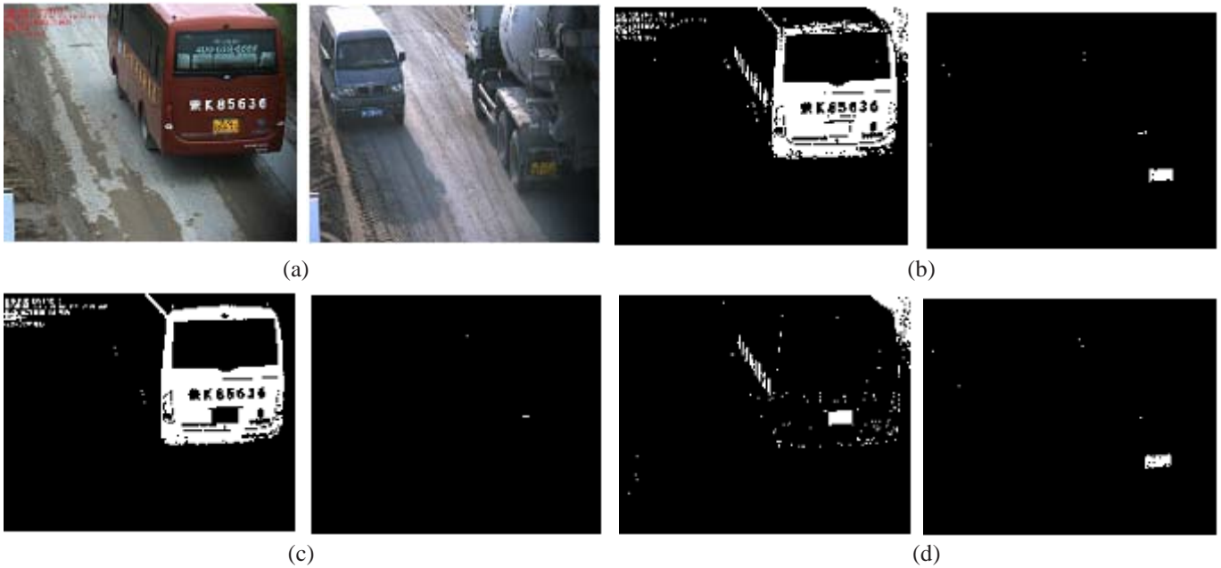
Figure 2 Extract yellow area: (a) The original image, (b) The yellow area of image with interference ( b_{im}(i,j) ), (c) The interference image ( a_{im}(i,j) ), (d) The the yellow area image ( c_{im}(i,j) )
