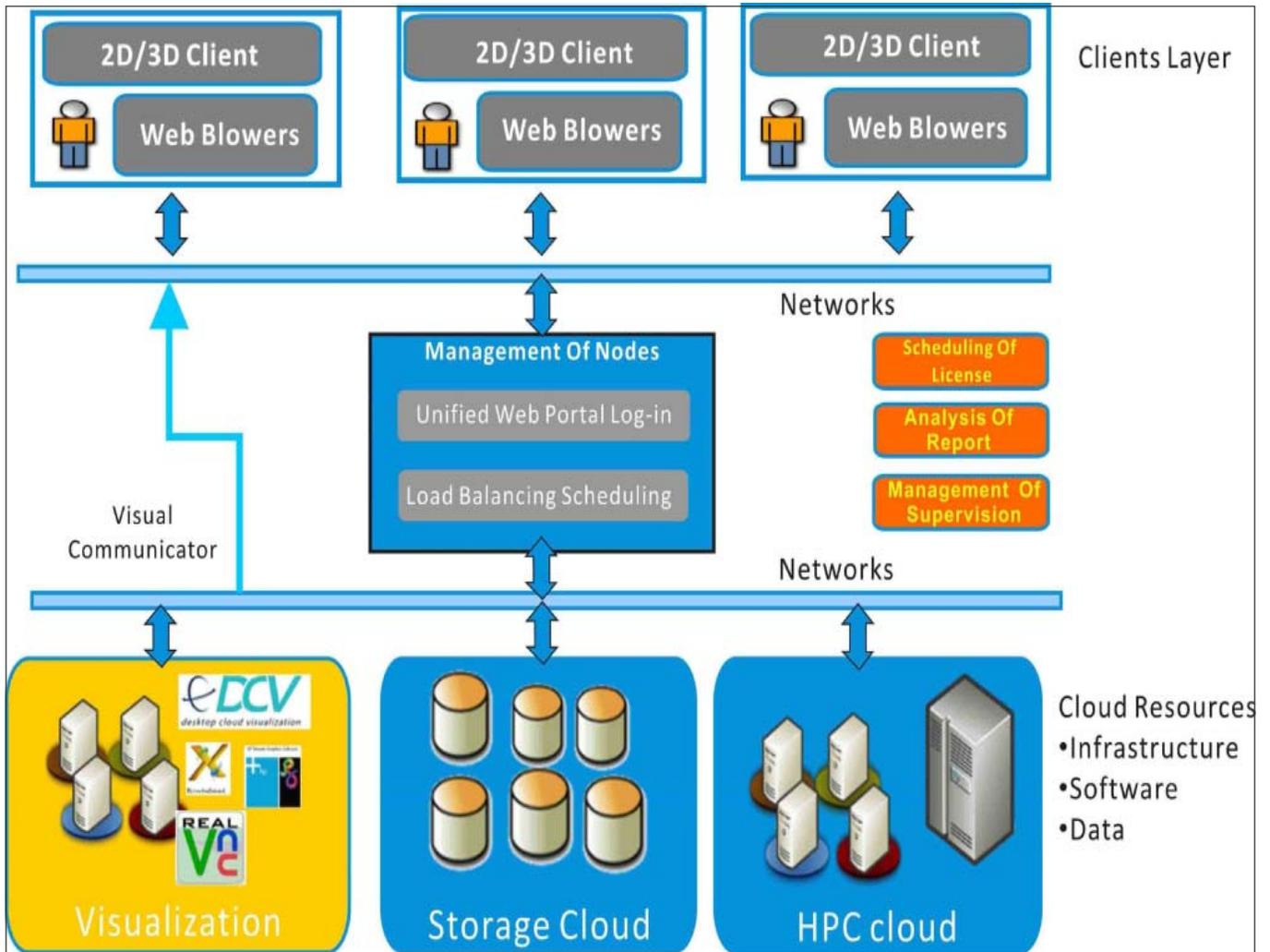
Figure 3. Overview of Self-service Cluster Remote Visualization Scheme
