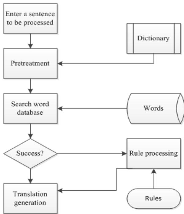
Figure 3. General procedure of MT System
