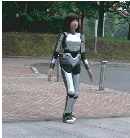
Figure 6. HRP-4C Humanoid: stable walking under linear inverted pendulum model [150]
