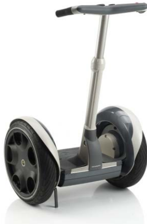
Figure 5. The Segway: A mobile wheeled inverted pendulum [139]
