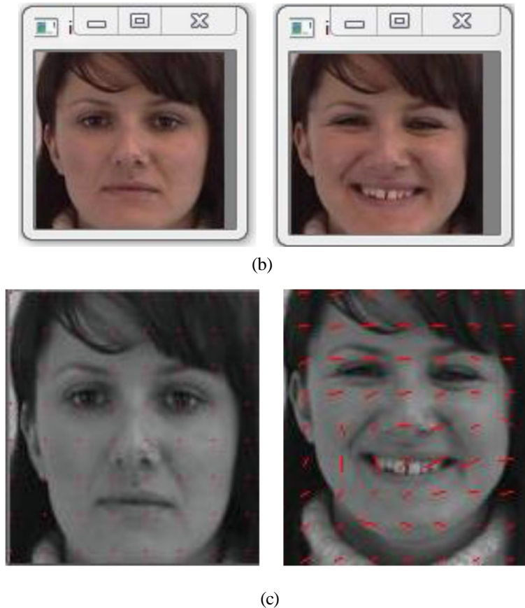
Figure 2. Face detection. (a) Source image, (b) Face detected, (c) Optical flow vectors
