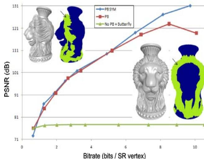
Figure 19. Bitrate-*PSNR* curves for the non-smooth region of the segmented Lion Head model, where the Butterfly prediction is used (without any wavelets) in the smooth region. The bitrate (reported in bits/SR vertex) corresponds to the bit allocation after quantization, with respect to the number of vertices in the SR non-smooth patch
