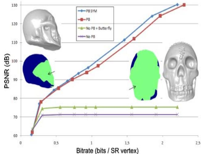
Figure 18. Bitrate-*PSNR* curves for the non-smooth region of the segmented Skull model, where the Butterfly prediction is used (without any wavelets) in the smooth region. The bitrate (reported in bits/SR vertex) corresponds to the bit allocation after quantization, with respect to the number of vertices in the SR non-smooth patch. 18
