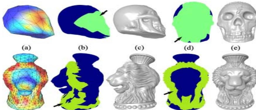
Figure 12. Illustration of the different steps involved in our classification and segmentation processes, on the 5<sup>th</sup> level of the Normal Skull model (top) and of the Lion Head model (bottom). (a) Averaging of the wavelet norms in the 5<sup>th</sup> level. The non-smooth region is depicted in green in the SR original model (b, d), whose features can be better appreciated with a Phong shading (c, e)
