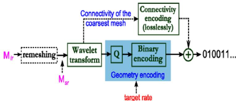
Figure 16. Main steps of a wavelet-based coder for SR meshes. Q stands for the Quantization step. The geometry encoding is generally done under a constraint which can be user-defined or automatic. This parameter can be a file size [5], a rate [8, 33], a reconstruction quality, etc
