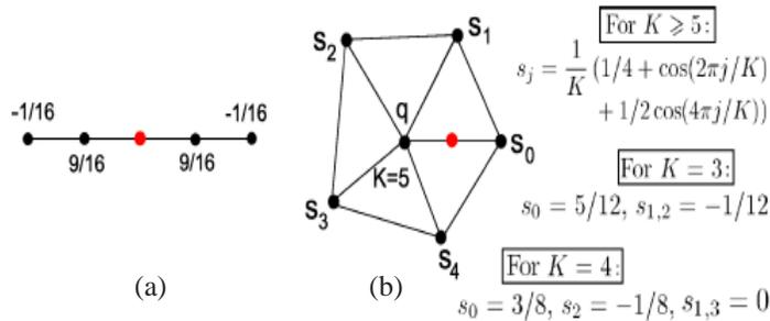
Figure 14. (a) Special Butterfly stencil used to predict the red vertex, situated on the mesh border (for non-closed 3D meshes); (b) Extension of the classical Butterfly stencil for extraordinary vertices (scheme proposed by Zorin et al. [26])
