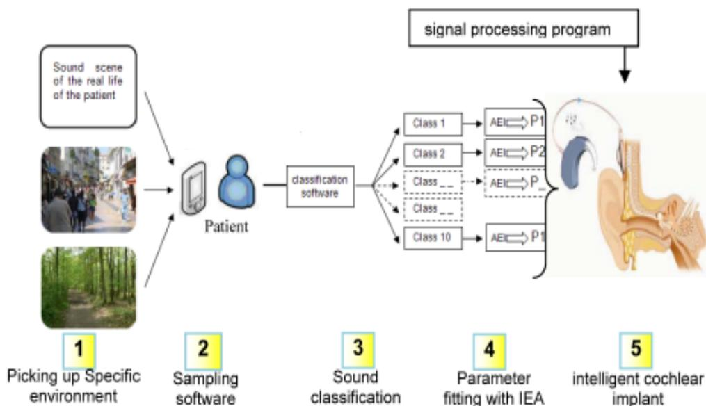
Figure 3. A block diagram of the proposed method for cochlear implant fitting
