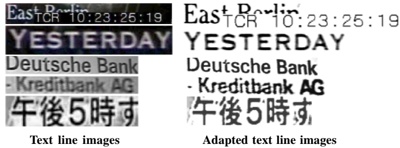
Figure 12. Exemplary resulting images of dynamic contrast/brightness adaption. Contrary to the originals, the revised images are suitable for being processed by OCR engines, as the background has been removed
