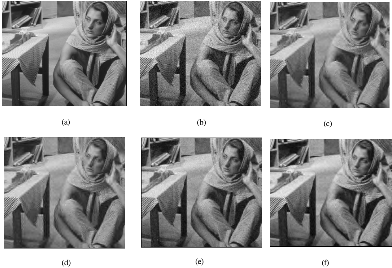
Figure 5. Denoising comparisons of Barbara image: (a) Original image, (b) Noisy image, (c) Global threshold denoising, (d) Maxmin threshold denoising, (e) BayesShrink threshold denoising, and (f) GMM
