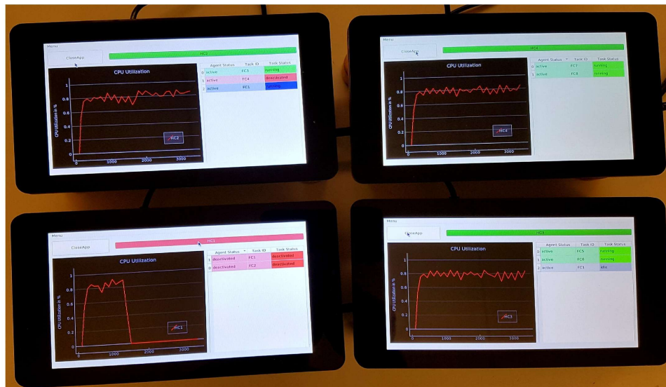
Figure 2. Our demonstrator setup consisting of 4 Raspberry Pis, which are connected over a switch and Ethernet links
