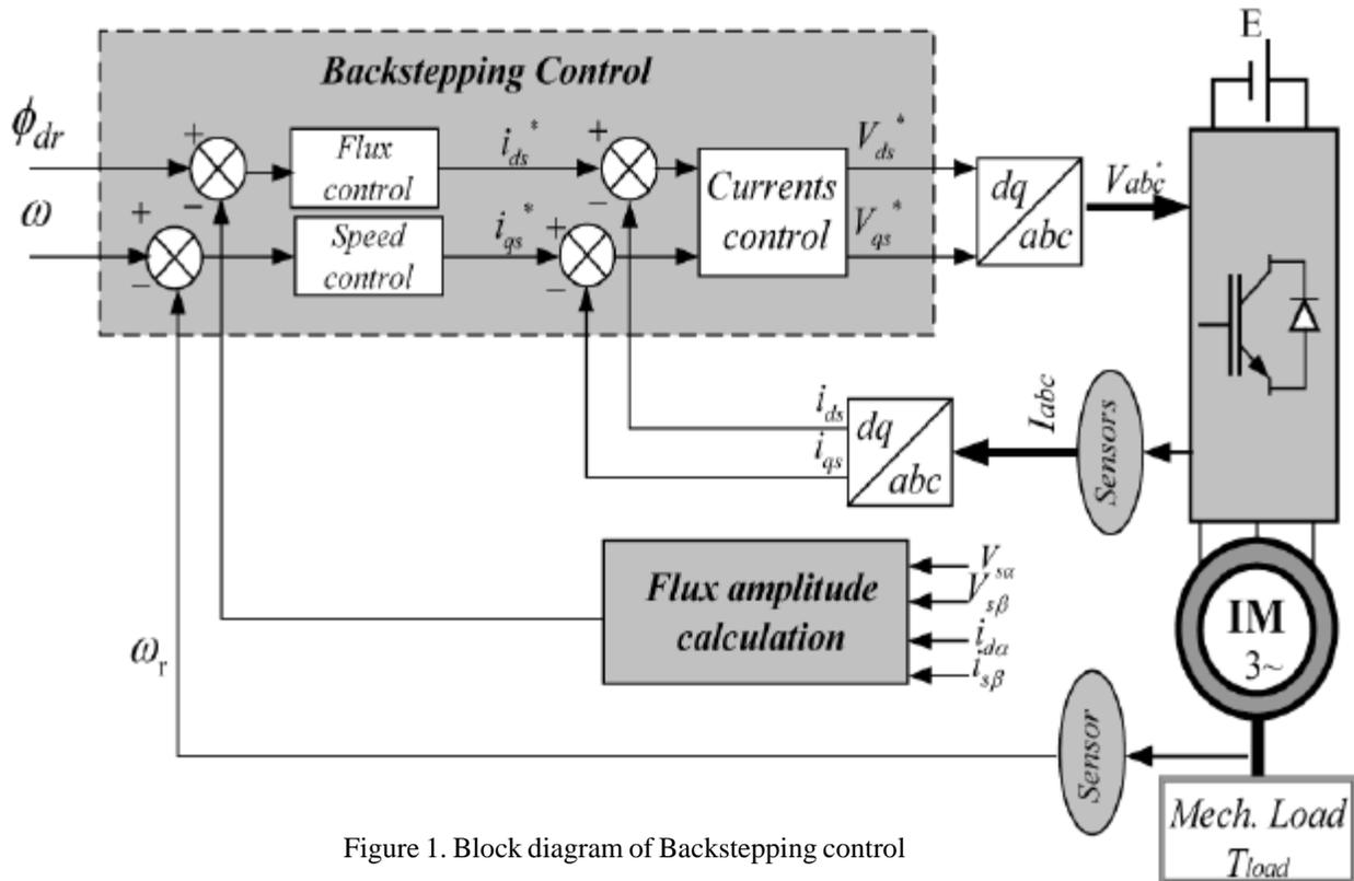
Figure 1. Block diagram of Backstepping control
