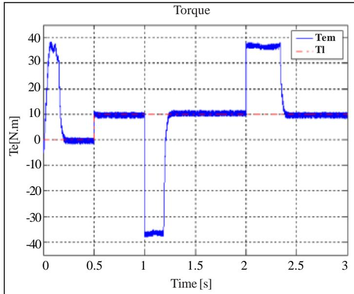
Figure 4. Torque response (second test)
