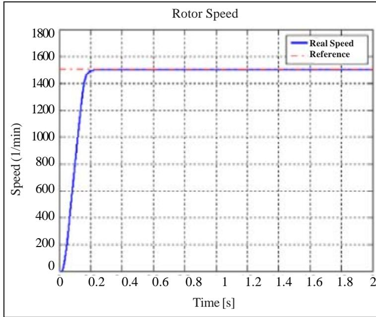
Figure 2. Simulated results to a step speed 1500tr/mn
