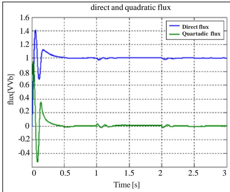
Figure 5. Direct and quadratic flux response
