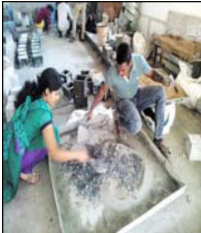
Figure 3. Batching And Mixing Of Concrete
