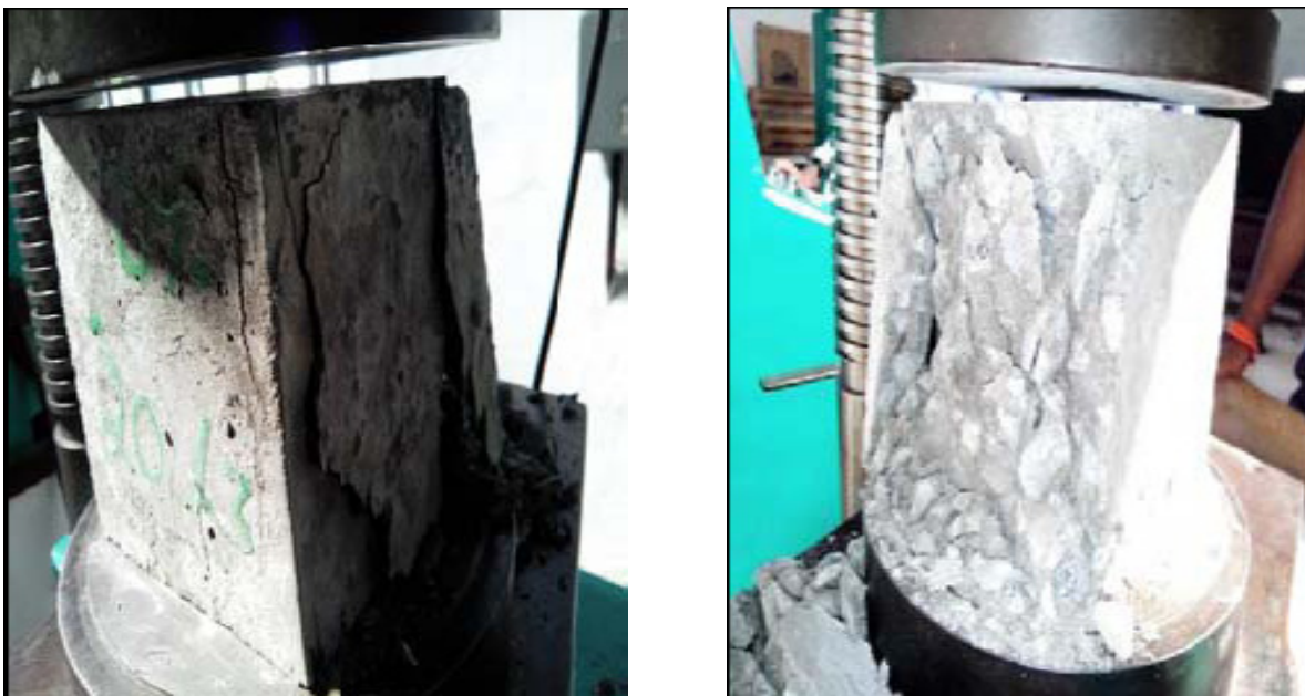
Figure 7. Failure of Cubes due to Compression Load
