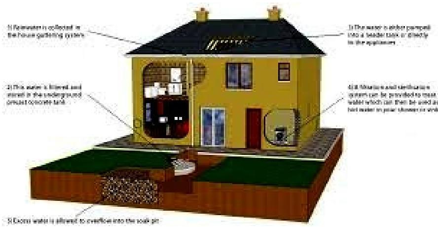
Figure 3. Use of rain water for garden and other uses
